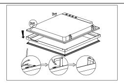
Step 2: Stand the 4 clasps of the lamp as shown and retate it 90 degrees to place the lamps into the outer frame. You can use hands (but be sure to wear the gloves) or use pliers and adjust the height of the clasps to the height of the outer frame to prevent the lamp from falling.
