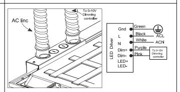
Step 4: Connect the AC Line accoding to the wiring diagram as shown in picture.
