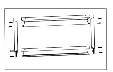
Step 1: Assemble and Fix the outer frame by screws as picture show.
