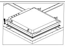
Step 3: Insert luminaire into T-bar ceiling grid. Secure safety cable to connection hole as needed to meet local seismic requirements. Safety cable and method of attachment to the building provided by contractor according to local building codes.
